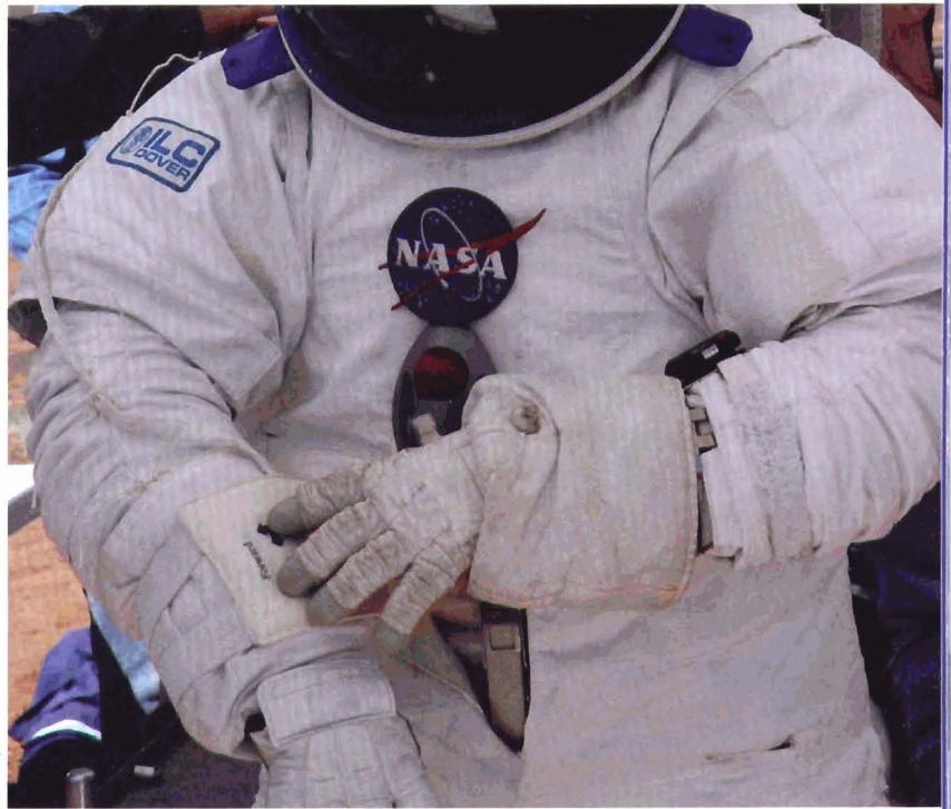
That’s an e-textile control pad on the astronaut’s arm.
